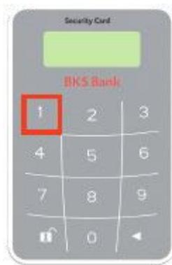
To calculate a new security code, enter “1” after “APPLI” appears on the display.
